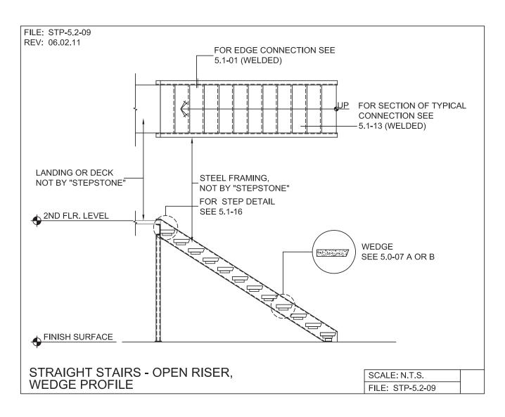
PRECAST CONCRETE TREADS AND LANDINGS SHOWN ON PLANS SHALL BE FROM THE LONG SPAN "STEPTREAD" SYSTEM BY "STEPSTONE, INC." OF GARDENA, CA FOR STEEL CONSTRUCTION. THE MANUFACTURER IS TO SUPPLY ALL PRECAST CONCRETE "STEPTREAD" SYSTEM PARTS, FEATURING BOTTOM WELD PLATES FOR WELD-ON CONNECTIONS. ALL REINFORCING AND CONNECTION PLATES WILL BE ZINC PLATED. ONLY ITEMS NOTED AS BY "STEPSTONE, INC." WILL BE FURNISHED BY "STEPSTONE, INC." SUCH ITEMS ARE TO BE INSTALLED BY OTHERS.
